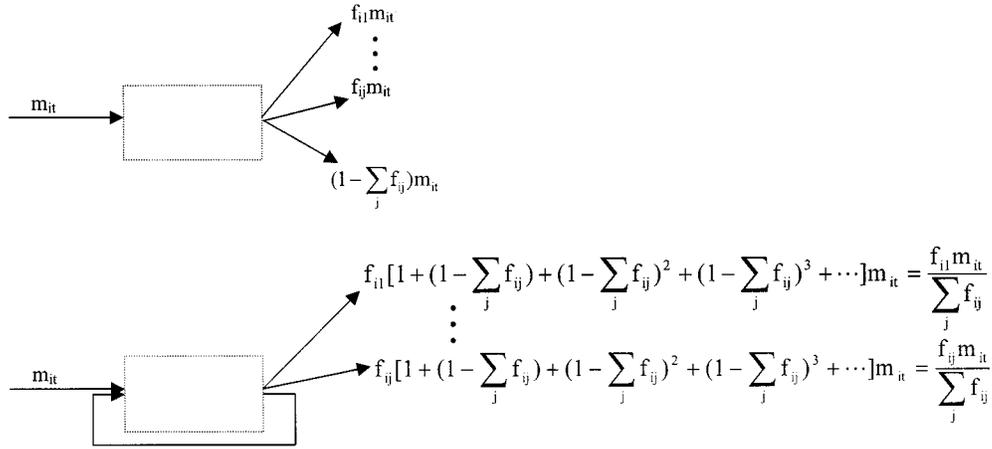
Fig. 2. Continuous reprocessing at one equipment step.
