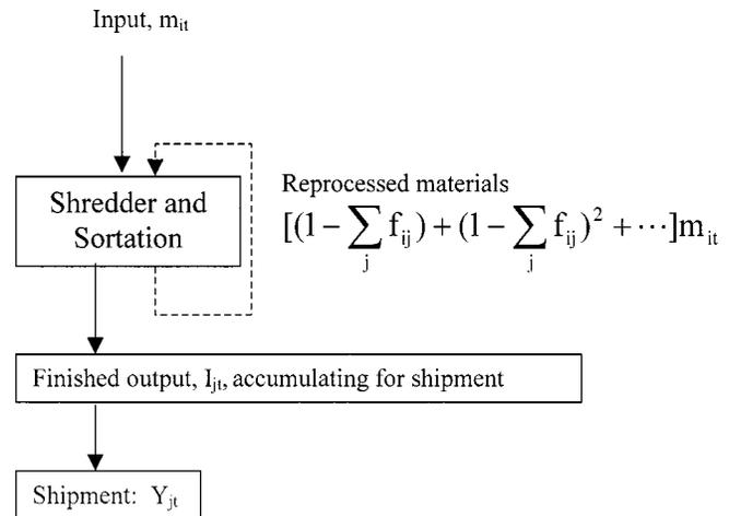
Fig. 1. Example of continuous reprocessing decision for bulk recycler.
