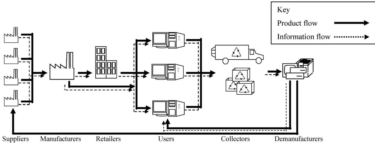
Figure 3. Future decentralized information flow for product environmental profile in which information is embedded in the product.
