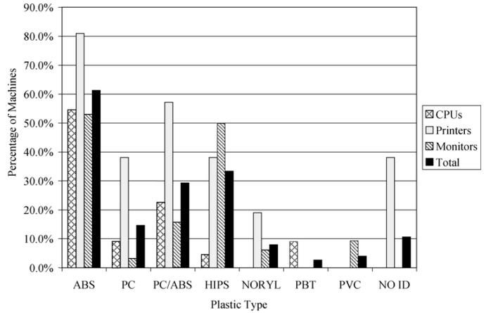
Fig. 2. Percentage of machines from which plastic pieces (>50 g) were disassembled for each plastic type.
