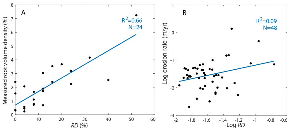
Fig. 2. Root density survey results. Root density measured by the root survey (*RD*) was strongly correlated to root volume density in soil pits (A), and was a weak but significant ( $p = 0.037$ ) predictor of streambank erosion rate (B).
