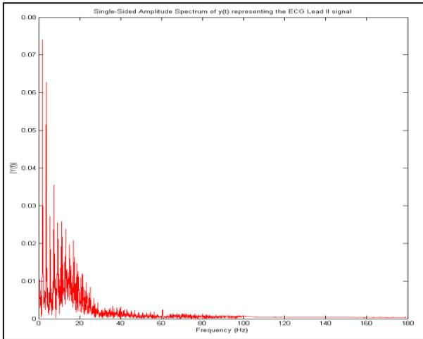
Fig. 9. Frequency spectrum of the baseband signal for the ECG Lead II signal.
