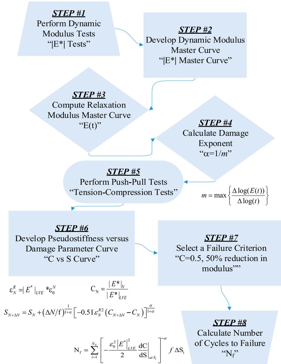
**Fig. 2.** Steps to perform viscoelastic continuum damage analysis.
