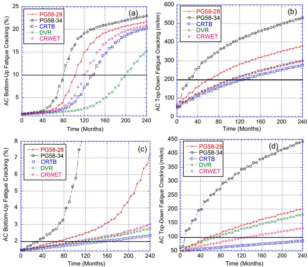
Fig. 5. Comparison of mixtures (a-c) Bottom-Up and (b-d) Top-Down fatigue cracking over time for thin- and thick-layered pavement structures, respectively.
