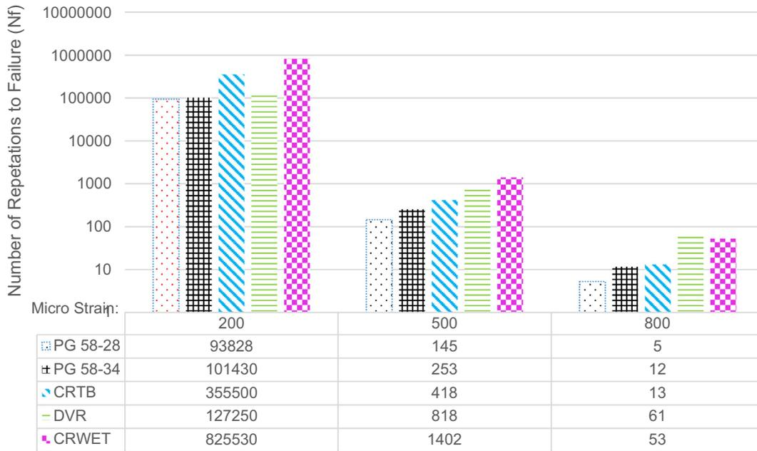
Fig. 3. PP-VECD fatigue analysis results for different microstrain levels at 20°C.
