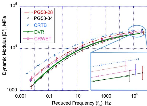
Fig. 1. Dynamic modulus ( $|E^*|$ ) master curves in a log–log scale at reference temperature of 21°C.
