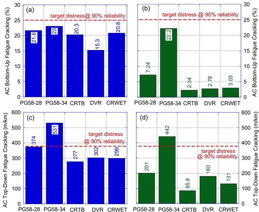
Fig. 4. (a) AC-BU cracking for thin- (b) AC-BU cracking for thick- (c) AC-TD cracking for thin- (d) AC-TD cracking for thick-layered pavement structures.
