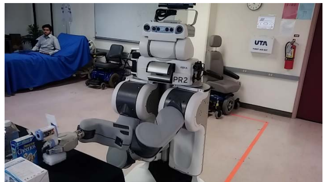
Figure 6. PR2 Robot Picks Up the Thermometer during an
