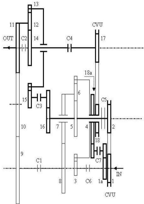
Fig. 1. A two-branch power split scenario, where C1..C7 : Clutches; CVU: Continuously Variable Units; 1, 2, 17, 18: Variable Pulleys; 3, 4..15, 16 : Gears, [3].
