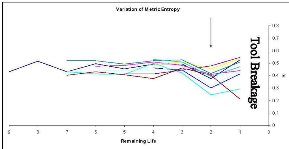
**Fig.2.** The metric entropy variations of all 10 drill bits.
