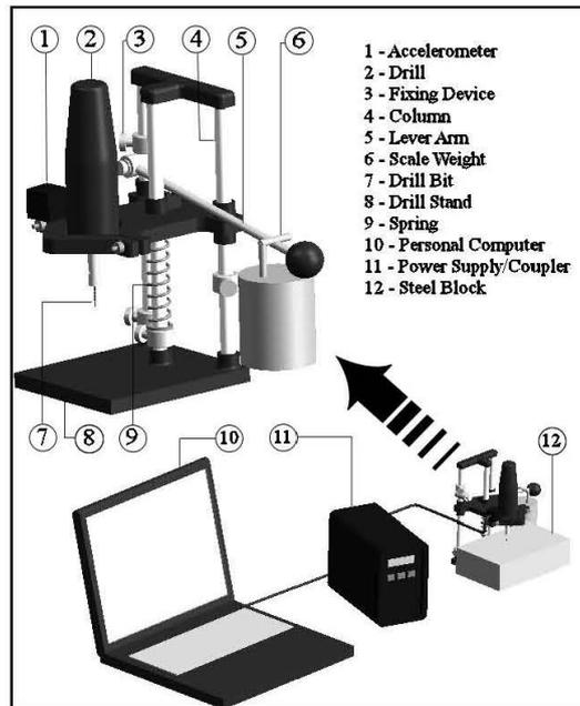
**Fig.1.** The schema of the test rig for drill bit breakage
