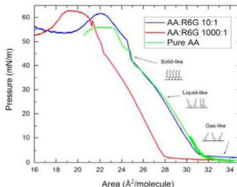
Figure 3: Isotherms of pure arachidic acid and arachidic acid doped with rhodamine 6G in 1:10 and 1:1000 ratios. Pure arachidic acid entered the solid phase at about 41 mN/m. The 10:1 R6G solution entered the solid phase at about 43 mN/m while the 1000:1 solution entered at about 46 mN/m.
