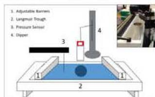
Figure 1: Kibron MicroTroughX and LayerXPro Dipper
