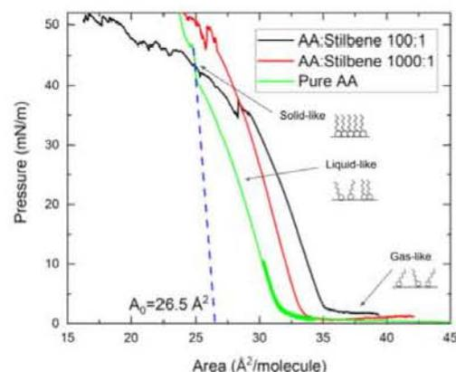
Figure 2: Isotherms of pure arachidic acid and arachidic acid doped with stilbene in 100:1 and 1000:1 ratios. Pure arachidic acid entered the solid phase at a pressure of about 41 mN/m while the 1000:1 stilbene solution entered the solid phase at about 45 mN/m. The 100:1 solution showed no evidence of a solid phase.
