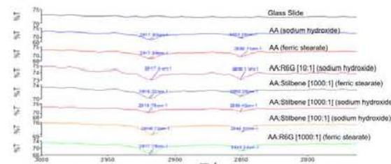
Figure 3 (above): FTIR of the LB films deposited onto glass slides. The way the film is prepared is in parentheses. The two peaks around 2917 cm<sup>-1</sup> and 2850 cm<sup>-1</sup> confirms the deposition of AA onto a slide. Figure 4 (right): The UV-Vis data of the stilbene slides prepared with ferric stearate shows negative absorbance.
