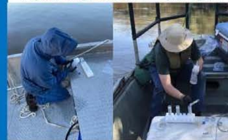
Ethanol is added to collected water samples from the Escambia River (left) and collected water is added to 50 mL tubes while sampling the Conecuh River (right)
